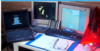
Radar scanners, AIS and data logging equipment employed in survey operations
